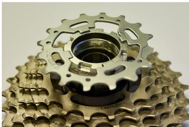
Remove the N3W adapter from the FW body and fit all sprockets except the two smallest sprockets.
