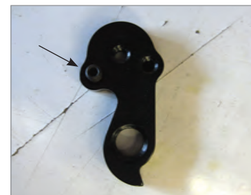
Figure 2 - Setscrew placement for vertical dropouts
