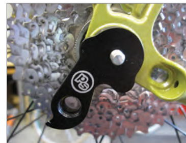
Figure 4 - Mounting for vertical dropouts
