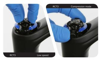
RCT3: Turn the low speed compression and compression mode knobs counter clockwise until they stop, to the full open positions.
