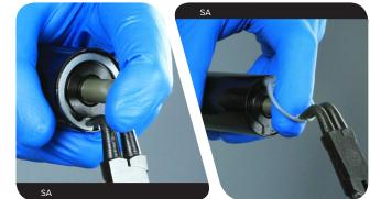
Place the tips of large internal retaining ring pliers into the eyelets of the retaining ring. Press firmly on the pliers to push the SA seal head into the upper tube enough to compress and remove the retaining ring. Slide the retaining ring onto your finger and release the air spring shaft.
