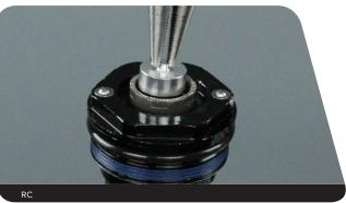
Use retaining ring pliers to install the inner retaining ring into the retaining ring groove.
