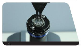
RCT3: Use needle-nose pliers to remove the low speed compression adjuster from the compression top cap.
