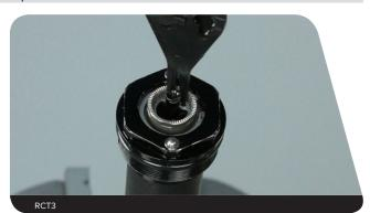
RC: Use small retaining ring pliers to remove the retaining ring from the bleed plug.
