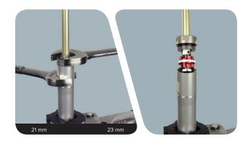
Remove the cartridge tube from the bicycle stand and pour the suspension oil into an oil pan.
