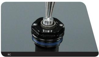
Use your fingers to install the bottom bolt into the rebound damper shaft, then pull down on the bottom bolt.
