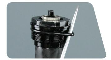
Lightly clamp the cartridge tube into a bicycle stand with the rebound damper shaft oriented upward.
