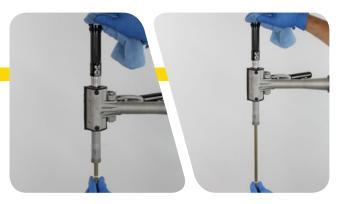
Fill the RockShox<sup>®</sup> Charger bleed syringe half full with 3wt suspension oil and thread the syringe and Charger hose fitting into the compression top cap assembly.
