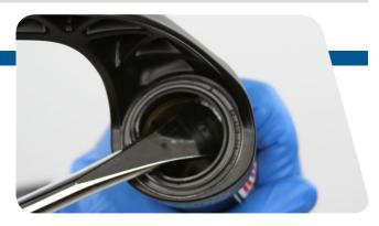
Stabilize the lower leg on a bench top or on the floor. Press down on the tire lever handle to remove the dust wiper seal. Discard the wiper seal.
