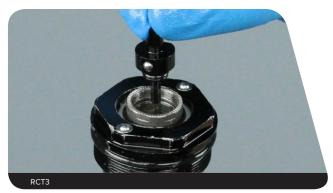
**RC:** Use needle-nose pliers to insert the bleed plug into the compression adjuster until it clicks into place.
