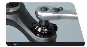
Dual Position Air<sup>™</sup>: Use a 10 mm socket wrench to loosen and remove the
