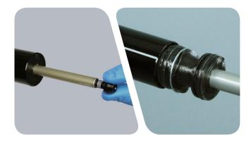
Spray isopropyl alcohol on the inside and outside of the upper tube and clean it with a rag.
