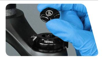
Use a small hex wrench to depress the Schrader valve and release all air pressure from the air chamber.
