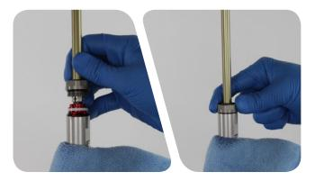
Place a torque wrench with a 23 mm crowfoot open end wrench on the wrench flats on the damper seal head. Place a 21 mm open wrench on the wrench flats of the cartridge tube.
