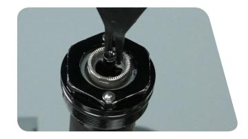
**Test the Bleed:** Rotate the compression adjuster cam **clockwise** until it stops. This is the locked position.
