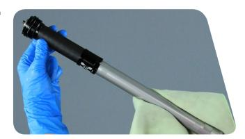
Insert and thread the Charger Damper into the top of the drive side upper tube.
