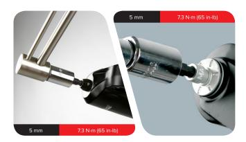
Install the rebound adjuster knob onto the rebound damper bottom bolt.
