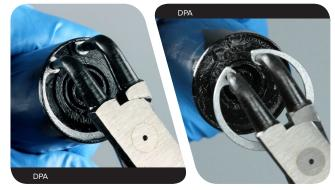
**Solo Air** $^{\rm \tiny NS}$ : Use a flat blade screwdriver to push the SA seal head tab under the retaining ring.
