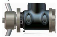
**3**. With a press tool, <u>GENTLY</u> press Non-Drive cup into Non-Drive side of frame so the O-ring just <u>BARELY</u> touches the side of frame. **DO NOT COMPRESS O-RING**
