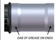
**3**. With the the O-ring and PF sleeve installed, put a dab of grease on the sleeve towards the ends of the cups.
