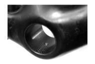
1. Remove the stock BB/bearing assembly so the Specialized Carbon frame shell is completely empty like the photo here. If any left over debris from prior BB, please clean out so frame shell is perfectly clean.
