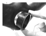
**2**. Put a tiny dab of grease on the provided Praxis Delrin PF cups. Then using your press tool, press one PF cup into each side of frame.
