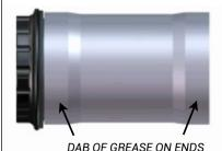
**3**. With the the O-ring and PF sleeve installed, put a dab of grease on the sleeve towards the ends of the cups.
