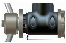
**3**. With a press tool, <u>GENTLY</u> press Non-Drive cup into Non-Drive side of frame so the O-ring just <u>BARELY</u> touches the side of frame. **DO NOT COMPRESS O-RING**
