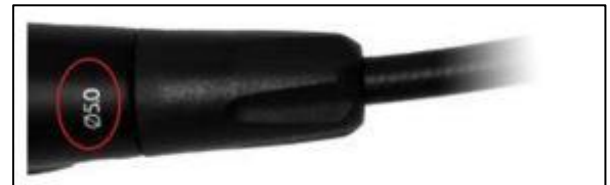
5mm oil hose symbol printed on some levers.
