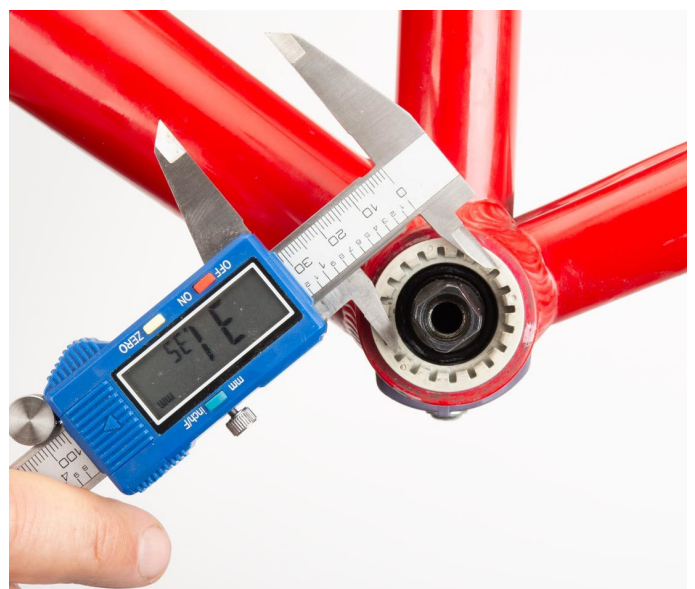
MEASURING THE MAJOR DIAMETER OF THE CUP
