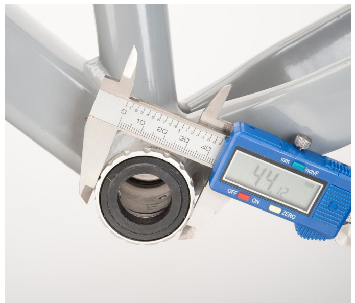
MEASURING THE MAJOR DIAMETER OF THE CUP
