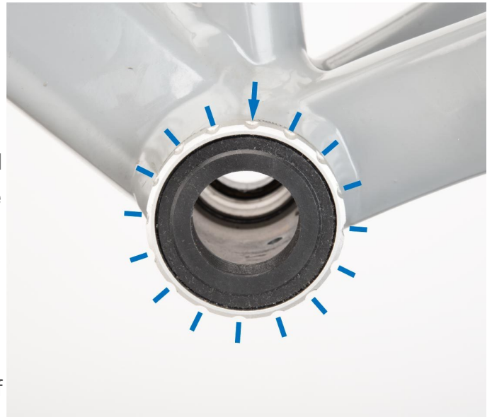
THIS CUP HAS 16 NOTCHES AS TOOL FITTINGS
