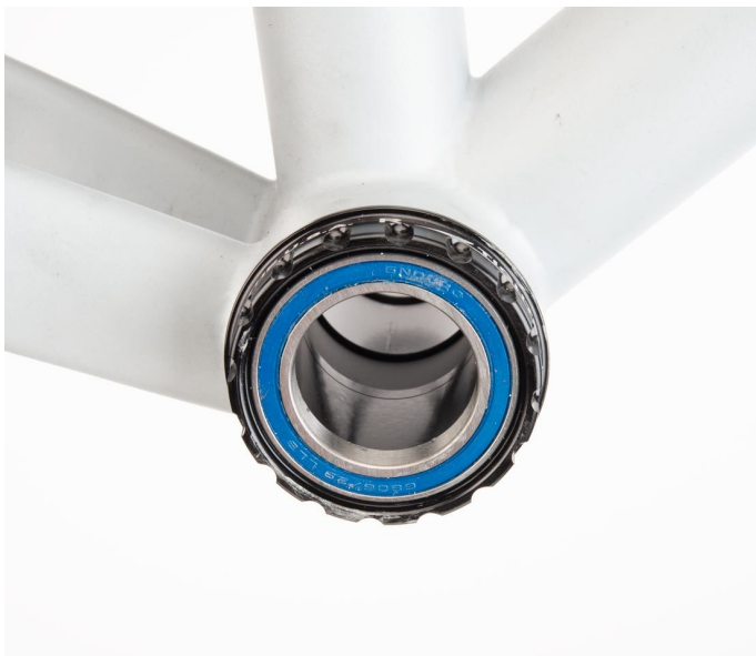
16 EXTERNAL NOTCHES, 52–54 MM OUTSIDE DIAMETER
