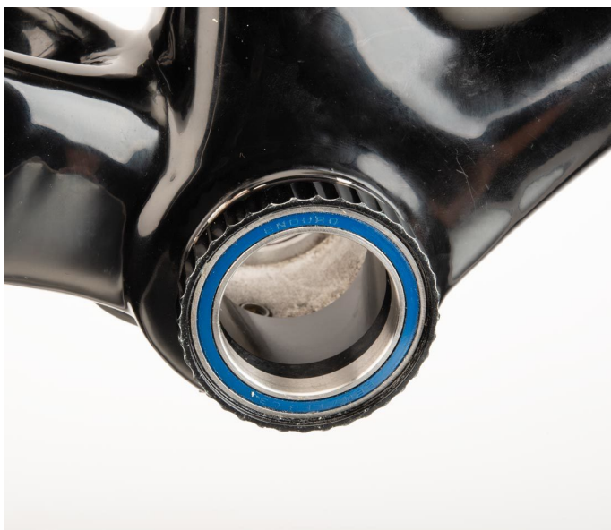
36 EXTERNAL NOTCHES, 51–53 MM OUTSIDE DIAMETER
