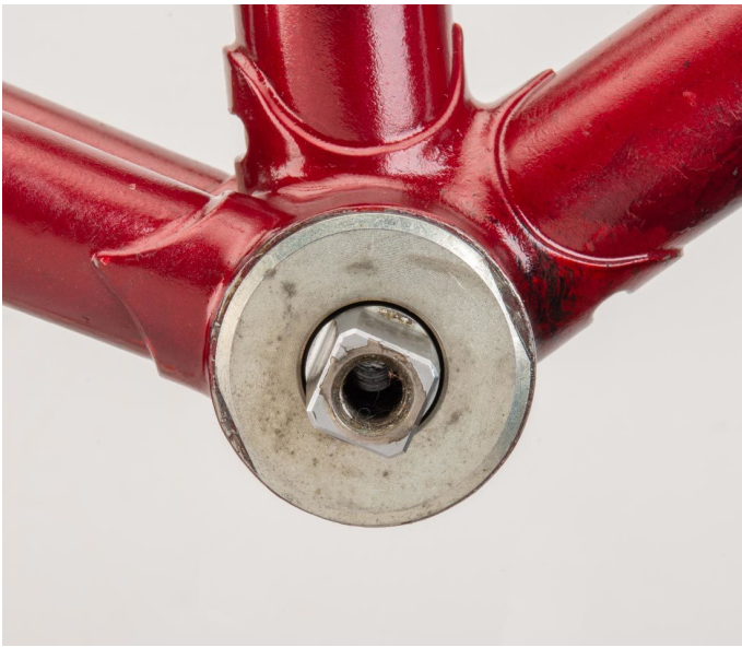
BOTTOM BRACKET CUP WITH TWO WRENCH FLATS
