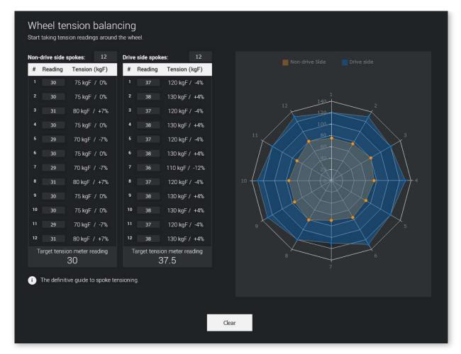
Move around the wheel and take readings for each side of the wheel at a time.
