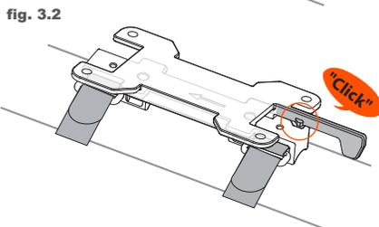
3. To attach bag, align the rails on bottom of bag with attachment, and slide forward. Bag is securely locked in when you feel a distinct 'click' (fig. 3.1, fig. 3.2).
