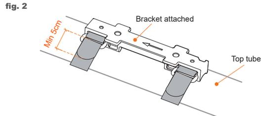
2. Wrap straps around tube, threading tongue through buckle. Join both ends of Velcro to fasten. Adjust as necessary. Tighten well, preferably with a 5 cm length of Velcro fastened. If straps are too long, trim with scissors (fig. 2).
