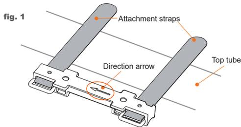
1. Attach bracket to top tube by seating the bracket rounded side down on the tube with direction arrow facing front of bike (fig. 1).
