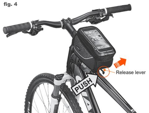
4. To release bag, push release lever firmly to the right, and slide bag rearwards (fig. 4).
