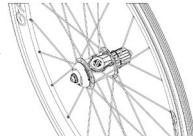
*When using on a Mountain Bike is recommended that the speed sensor be mounted on the rear hub.*
