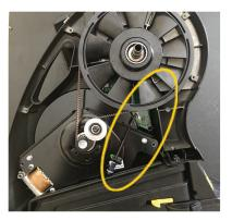
Lift the case of the Hammer to gain access to the tension screw, you can gain access to the tension screw port by opening up the leg.
