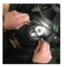
To install the new belt slide the new belt between the two pulleys.
