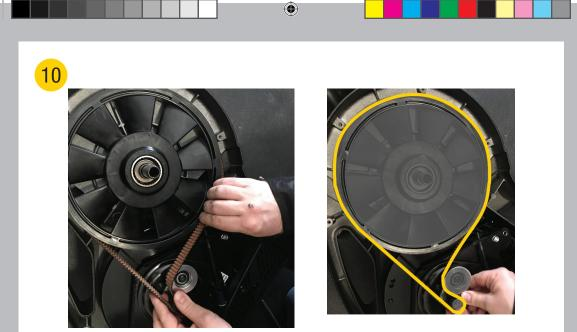
The path for the belt is around the large flywheel and then in between the two pulleys.
