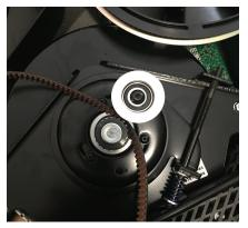
Slide the belt between the pulleys and remove the belt.
