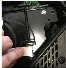
Check the distance between the two washers with the provided measuring gauge. It should be 3/4in.
