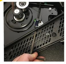
Tighten the tension screw.
