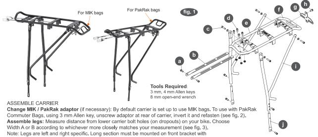
its three bolt holes facing out (see fig. 1). For bikes with wide seat stays: attach legs to outside leg bracket with bolt head on outermost hole (see fig. 3). For bikes with narrow seat stays: attach legs to inside of inner leg brackets with bolt head on innermost hole (see fig. 3).
